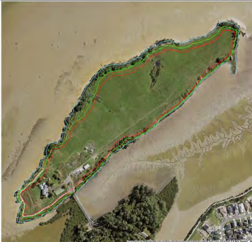
Figure 47: Aerial photo of Pararekau island – Manukau Harbour (coloured lines showing area susceptible to coastal erosion or instability over varying timeframes) (Source: Auckland council)
