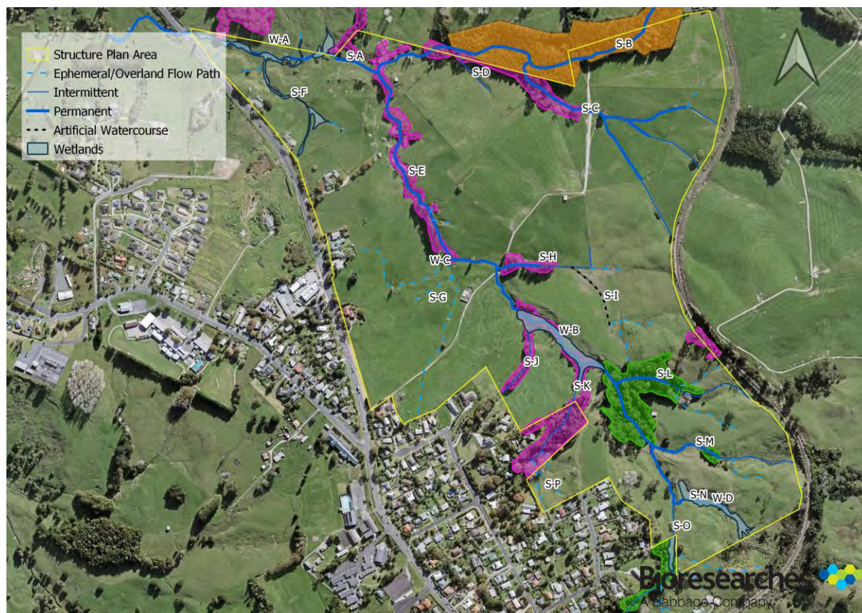
Figure 11. Freshwater features identified on site, including the permanent, intermittent or ephemeral status of streams, and wetland areas.
