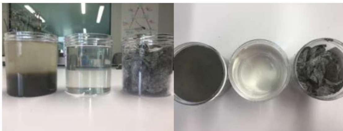
Picture showing incoming sludge on the left, residue clear water following filter in the middle and sludge converted to biosolid on the right
