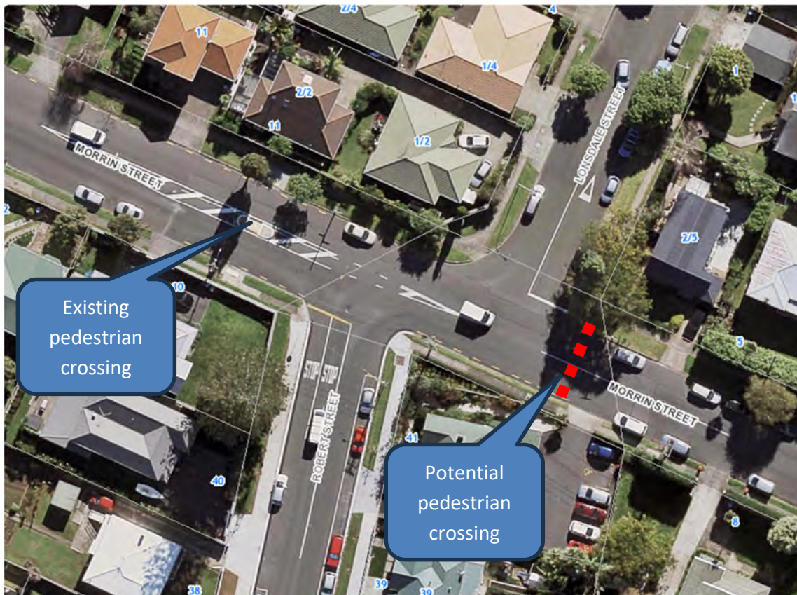
Figure 6: Morrin Street / Lonsdale Street / Robert Street staggered intersection
