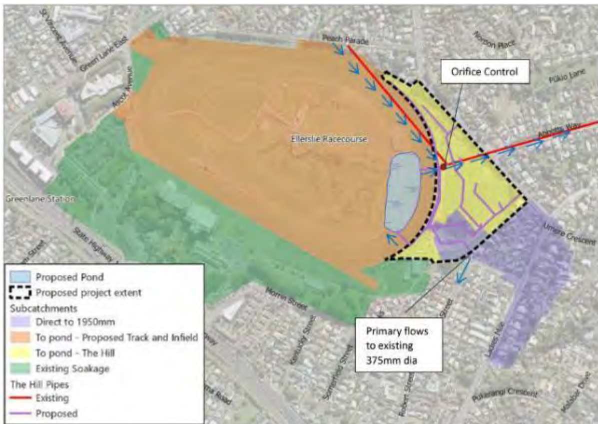
Figure 3. Diagram of the drainage pattern of the Ellerslie Racecourse and The Hill, source SMP by Woods, 22 September 2022
