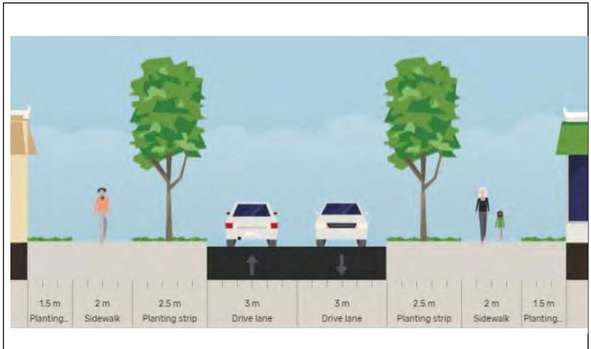
Figure 9 – Local Road Cross Section
