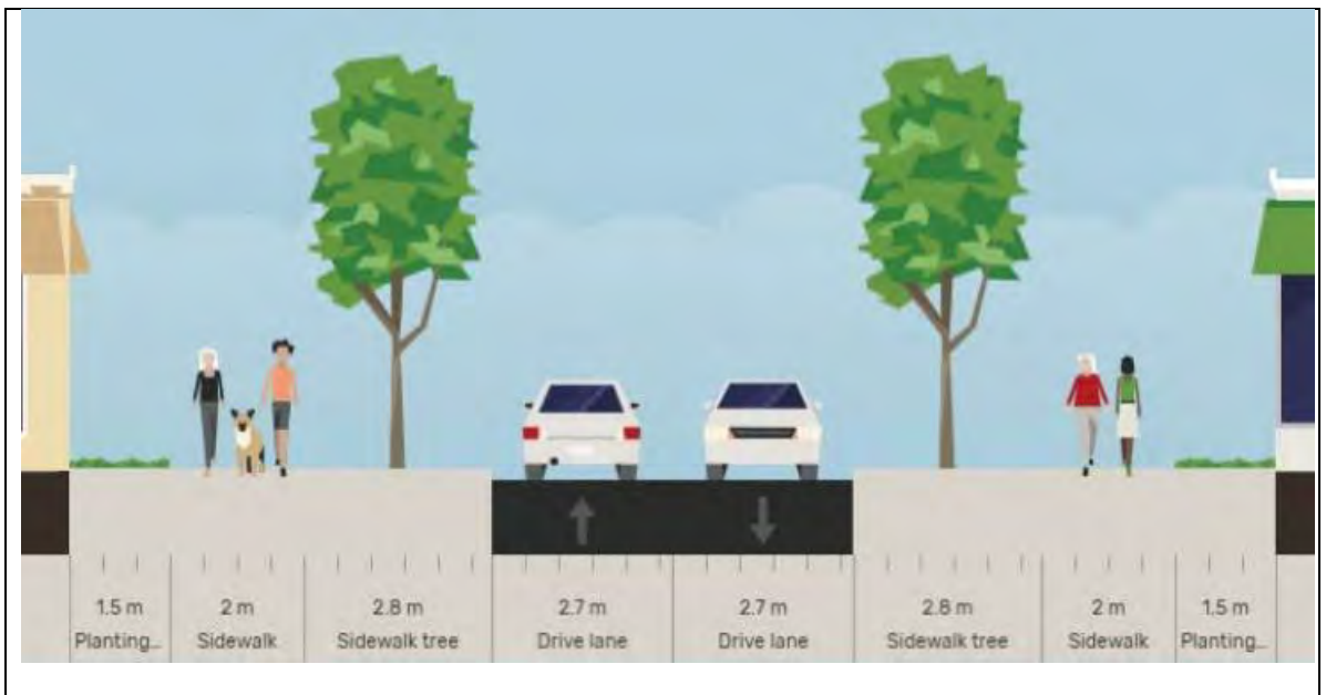
Figure 8 – Minor Road Cross Section
