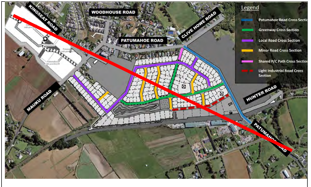
Figure 5: Roading Hierarchy – Sub-precinct E
