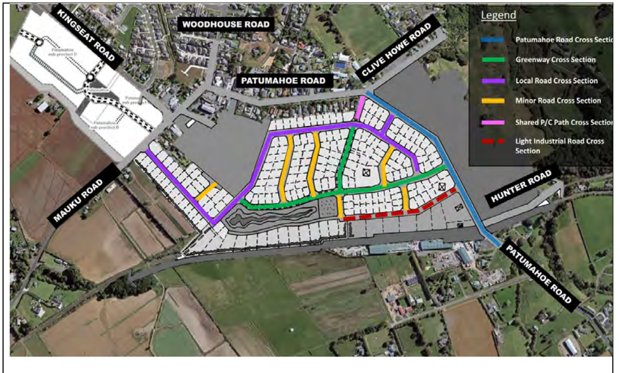
Figure 5: Roading Hierarchy – Sub-precinct E
