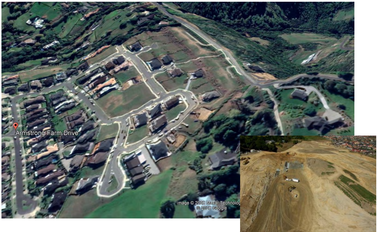
Inset 8: Typical outcome of geotechnical land stabilisation works permitting safe urbanisation (Armstrong Farm Drive, built on a landslide 15 years ago involving shear keys and drainage, located near the case study area presented above) – extracted from Google Earth database looking north, with inset same site actual aerial photograph of large scale shear key and drainage during construction looking south
