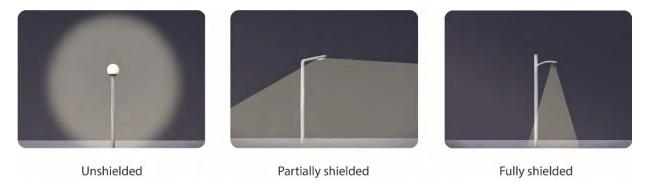
Figure 11 Lights should be shielded to avoid lighting anything but the target area or object. Figure adapted from Witherington and Martin (2003)<sup>3</sup>.
