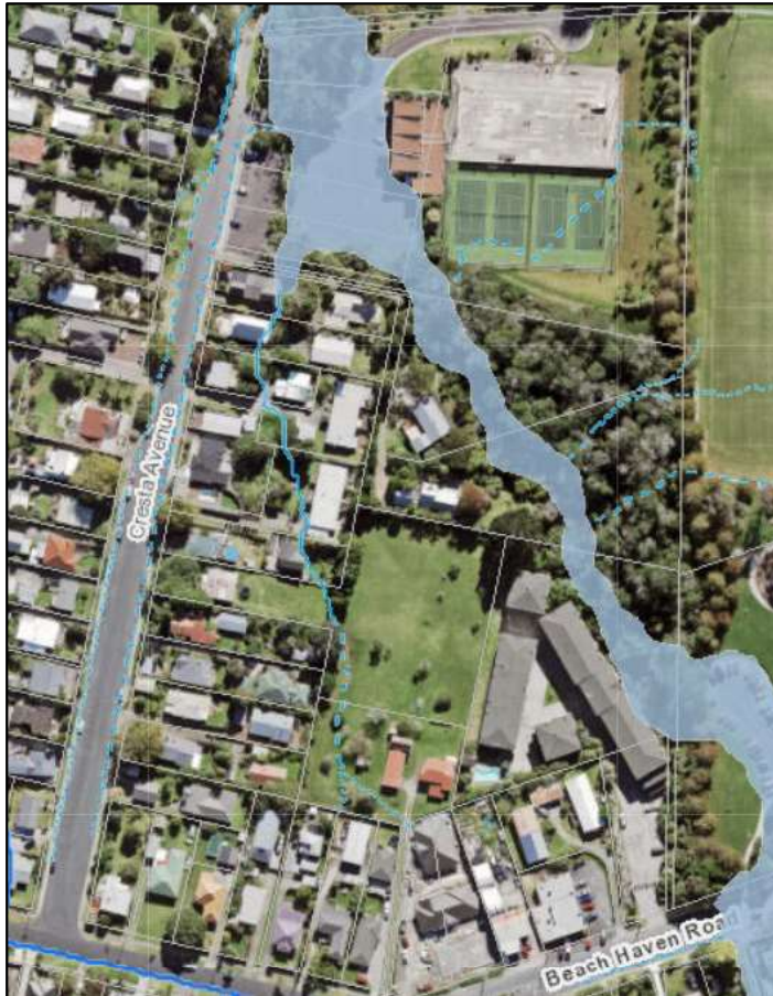
Figure 1: Overland flow paths and flood plain
