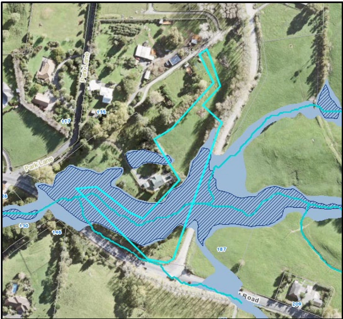
Figure 4 – Flood Plain and Flood Prone Areas as identified on Auckland Council GeoMaps (accessed 5 July 2023).
