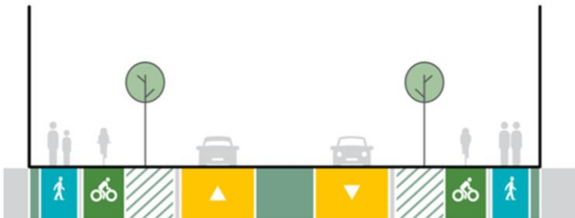
Figure 3: Woodcocks Road Indicative Cross-Section
