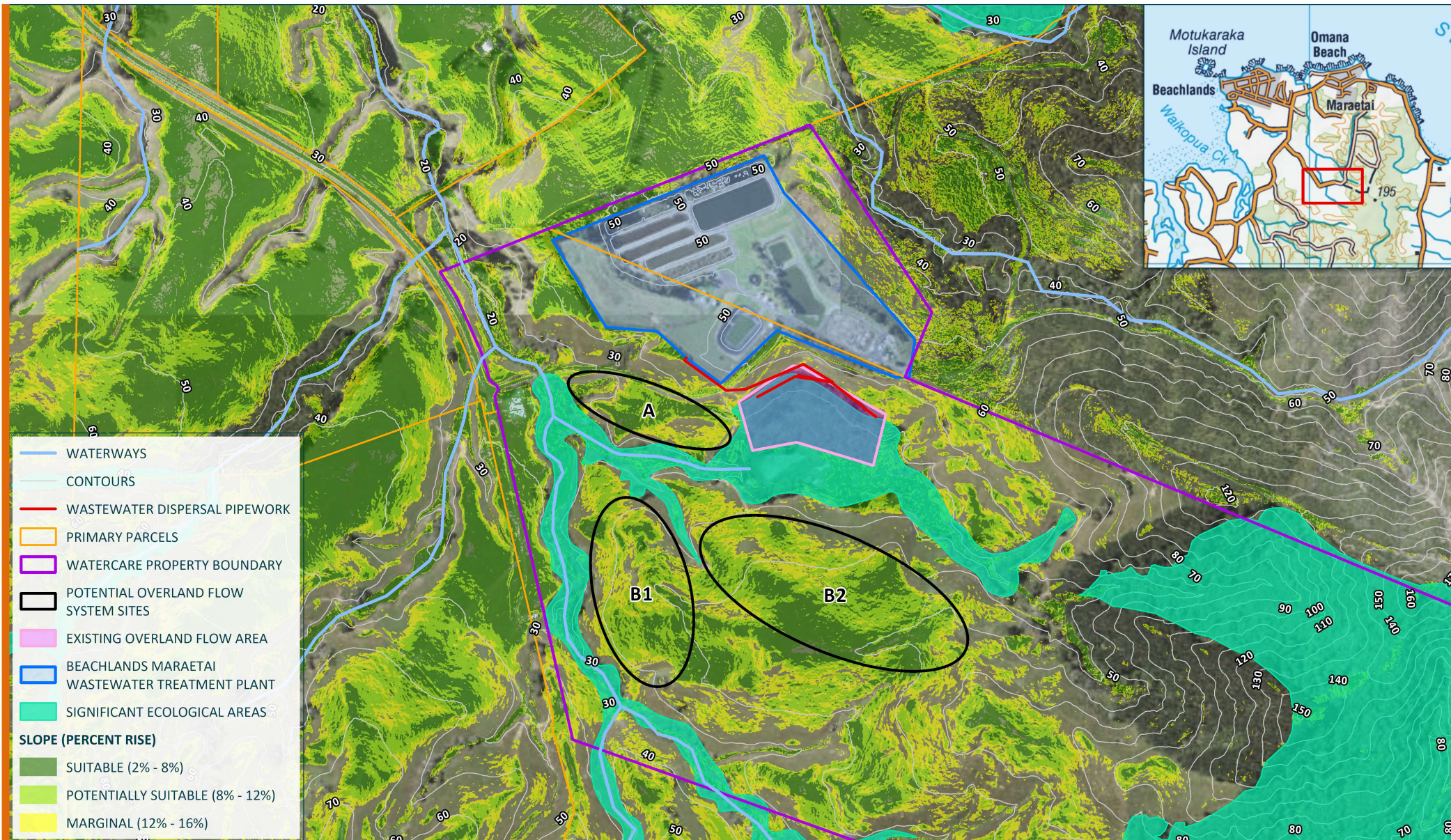
FIGURE 1: SUITABLE LAND AREA FOR AN EXPANSION OF THE BEACHLANDS WWTP OVERLAND FLOW SYSTEM
