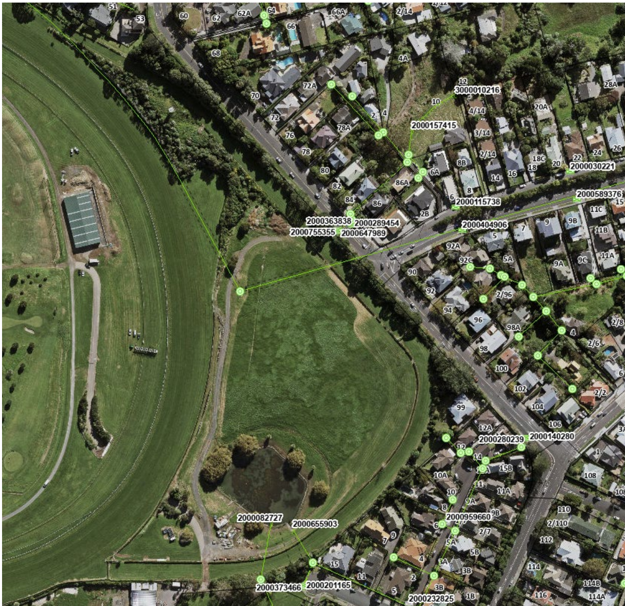
Figure 7: Remuera Precinct – Existing Stormwater Lines
