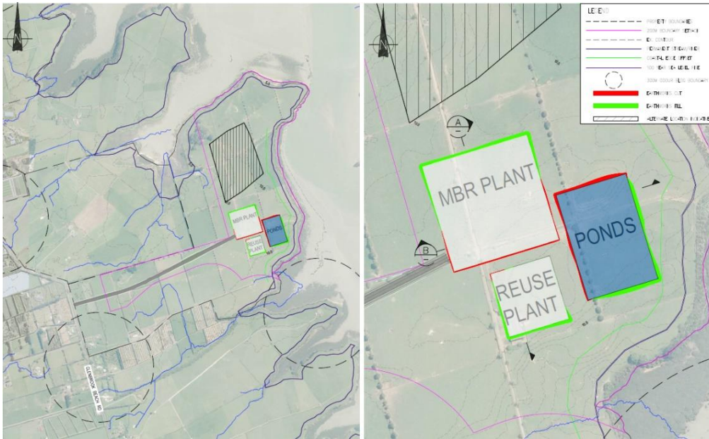
Figure 11: Site S indicative site layout (refer to Appendix D for more detailed plans). Hashed area shows possible alternative WWTP location, dashed circles show 300m from existing residential dwelling.
