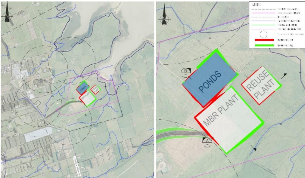
Figure 13: Site T indicative site layout (refer to Appendix D for more detailed plans). Dashed circles show 300m from existing residential dwelling.
