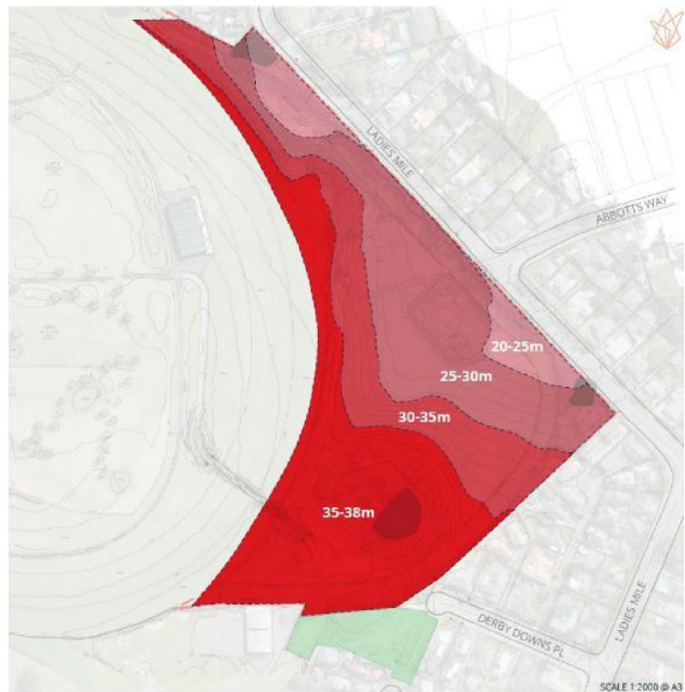
Figure 6: Diagram that indicates the maximum Building Height Range above ground (approx.) due to Volcanic Viewshaft
