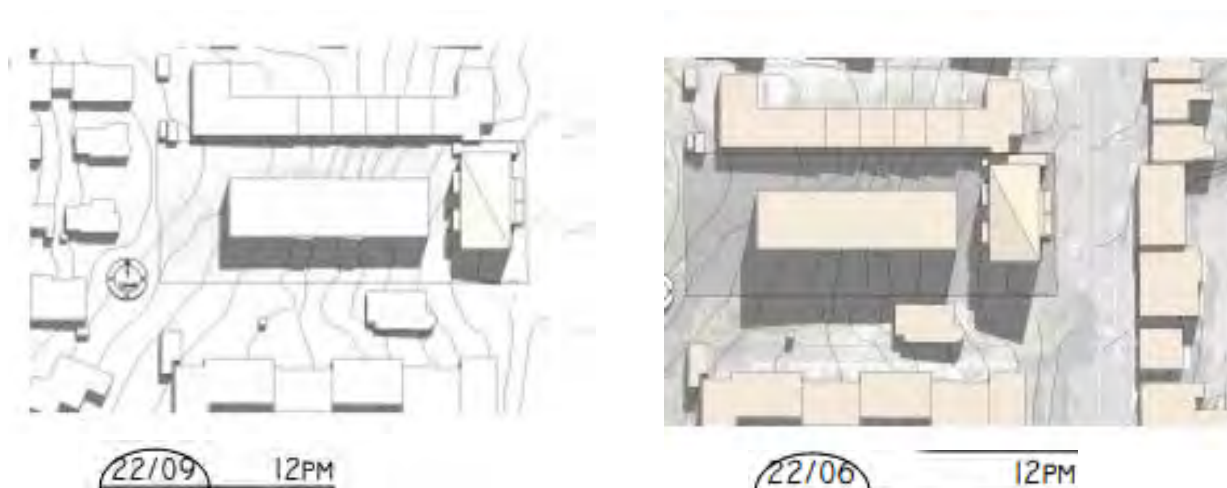
Figure 6 The shadow diagrams for this HIRB complying three storey apartment building in the THAB zone show the extent of shadow on the adjoining site at the equinox (22 Sept) and winter solstice (22 June).
