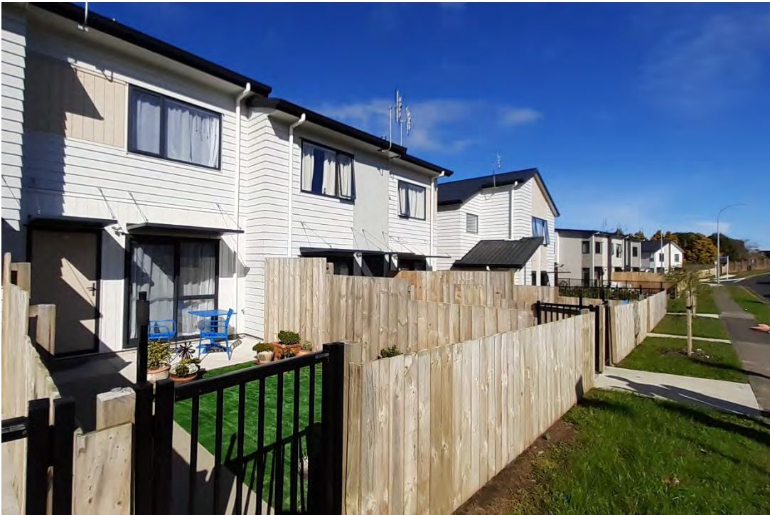
Figure 15: The 6m x 4m principal living outlook space depth and the 20m 2 outdoor living space orientated for sunlight are located together to create a spacious and healthy living area in this development.
