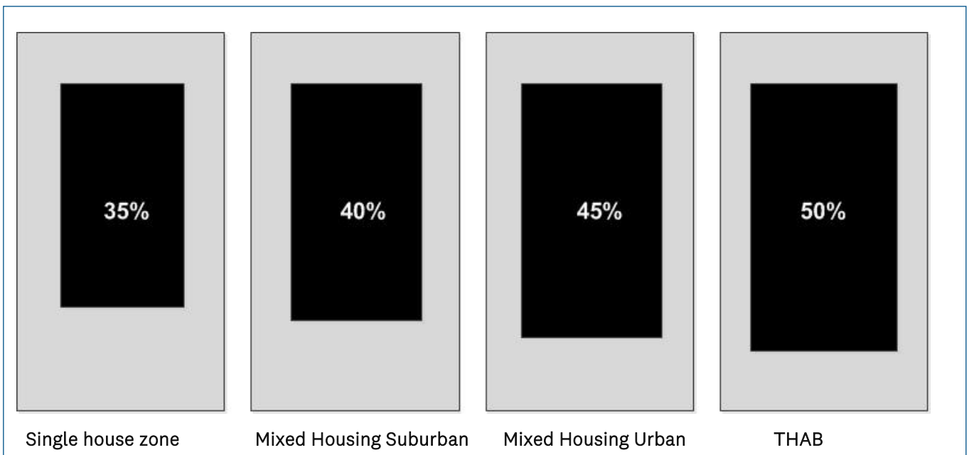
Figure 7. This diagram shows the percentage of building coverage (black area) for each residential zone applied to a theoretical 600m 2 site with an 18m site width and 33m site depth (space around the building is shown by the grey area). This illustrates the relative difference in building to open space ratio between the zones enabled through the building coverage standard.
