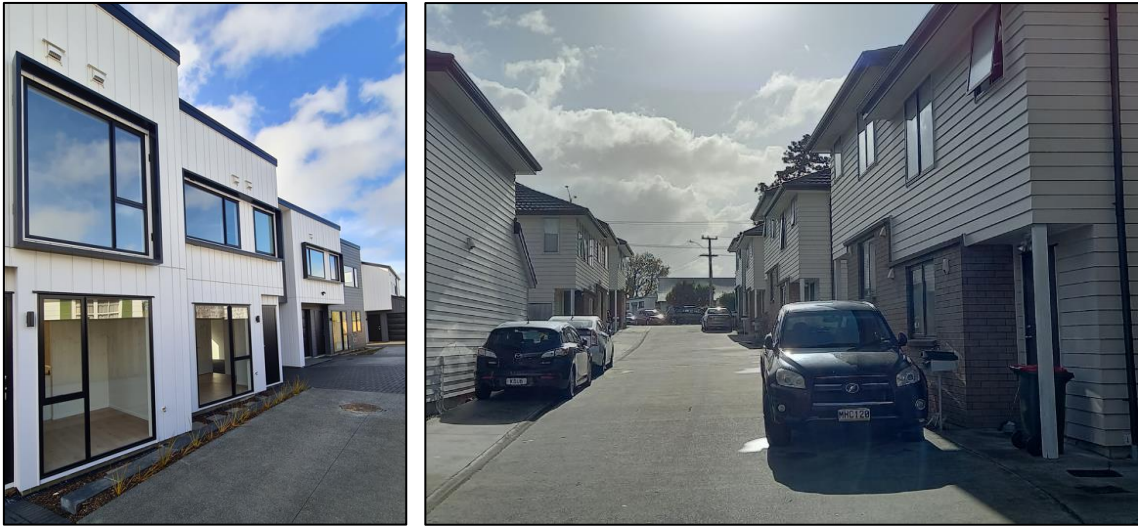
Figure 24: Two examples of no setback between the private vehicle accessways and adjacent dwellings
