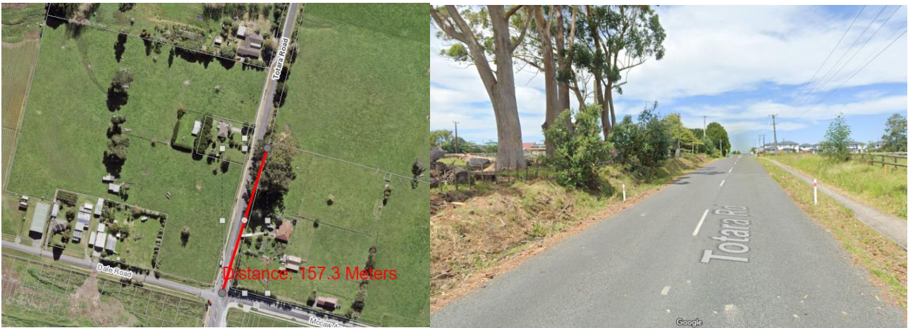
Figure 1.13 Sightline for the southern local road intersection with Totara Road, adapted from Council GIS and Google Streetview
