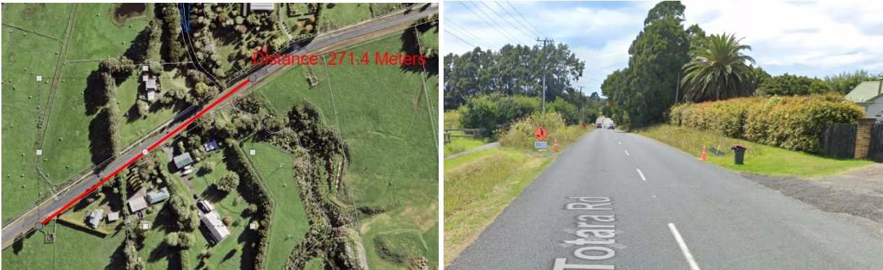
Figure 1.16 Sightline 2 for the northern roundabout with Totara Road, adapted from Council GIS and Google Streetview
