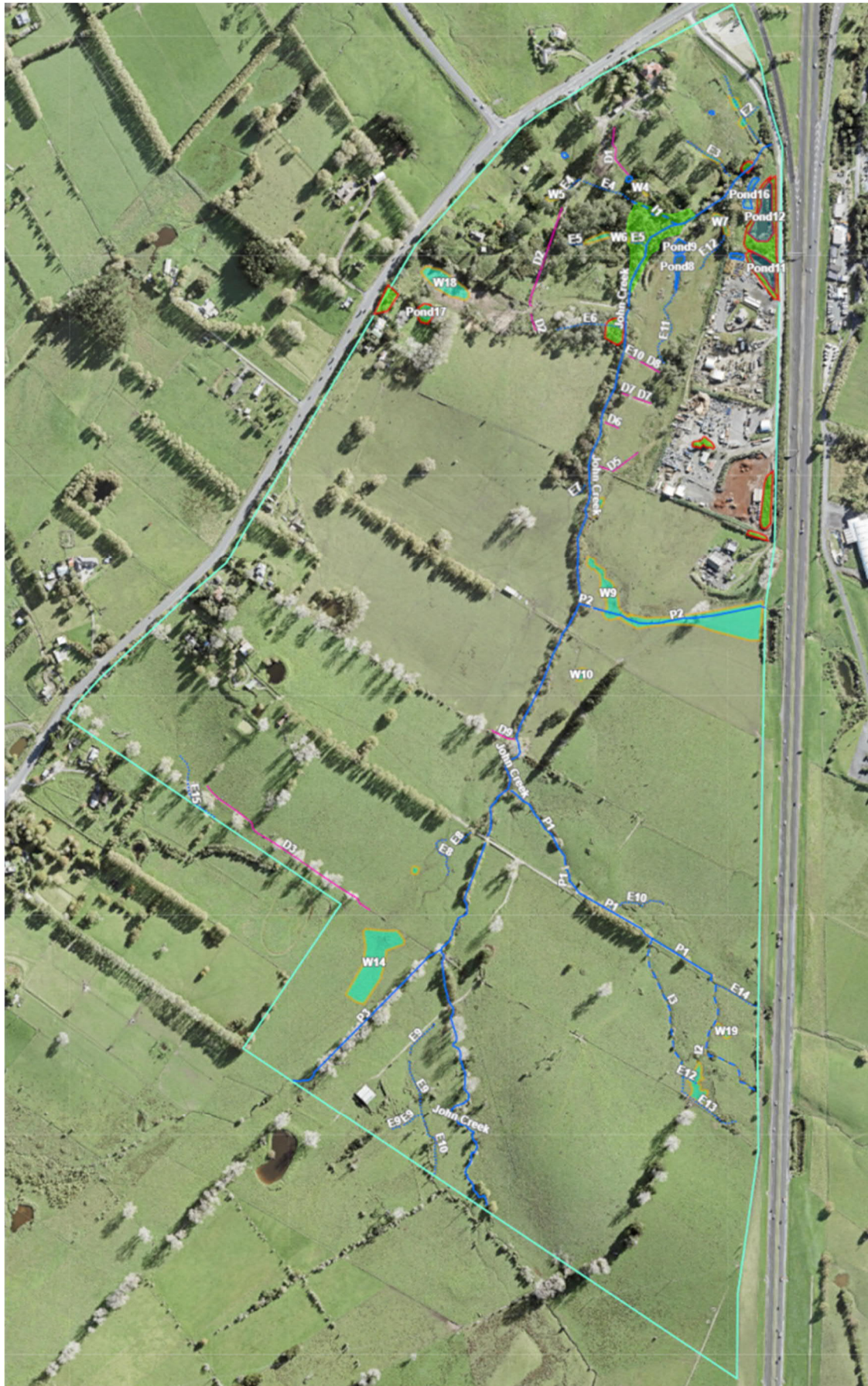
Figure 2. Watercourses and ponds at the site. Permanent stream (solid blue line), intermittent stream (dashed blue line), ephemeral flow path (dotted blue line), drain (solid purple line), pond (blue polygon with orange outline), and site boundary (turquoise line).
