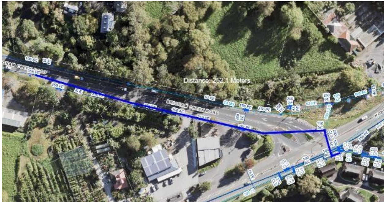
Figure 4 – Section of 150mm AC pipe to be upgraded in Brigham Creek Road.
