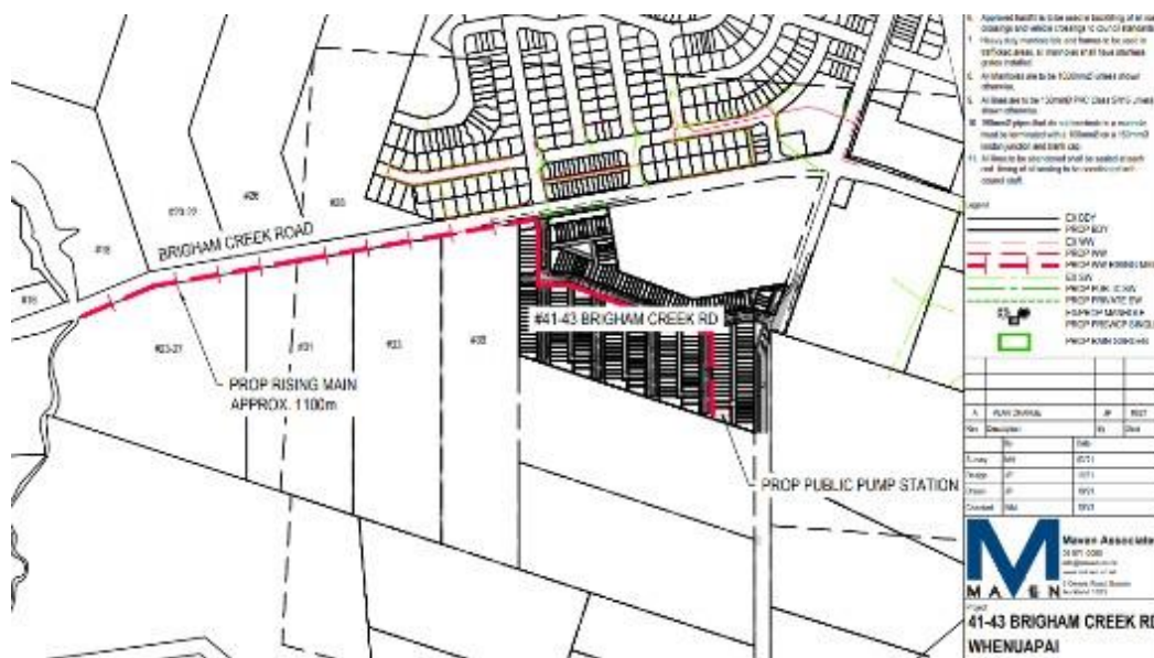
Figure 7: Plan Change 86 – Proposed Wastewater Ring Main Overview Plan
