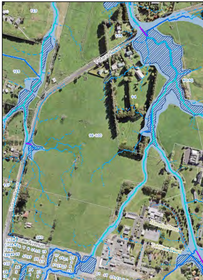
Figure 3: Overland Flow Paths and Flood Plains (Auckland Council GeoMaps 3.8°C increase due to climate change)
