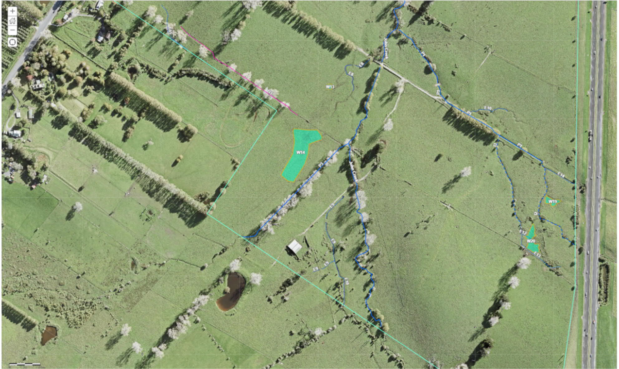
Figure 5. Watercourses across south portion of the site. Permanent stream (solid blue line), intermittent stream (dashed blue line), ephemeral flow path (dotted blue line), drain (solid purple line), pond (blue polygon with orange outline), and site boundary (turquoise line).
