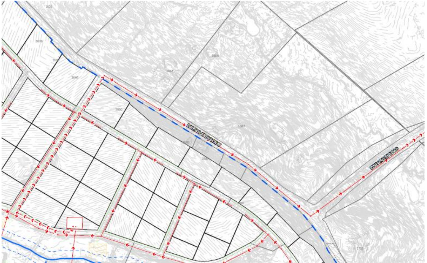
Figure 4: Proposed Wastewater alignment
