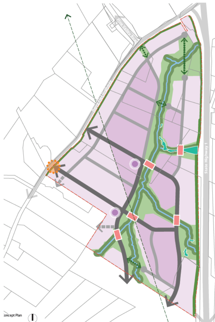
Figure 2: Development Concept Plan prepared by Barker & Associates. Purple(s) proposed light industrial, green proposed public open space and exiting waterways.
