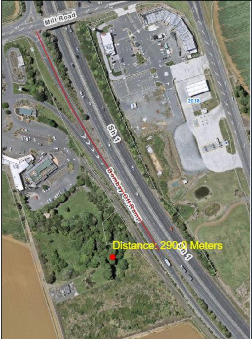
Figure 2 - Illustration of 290m distance between the stop line and the merging line of the left turn bypass onto Mill Road
