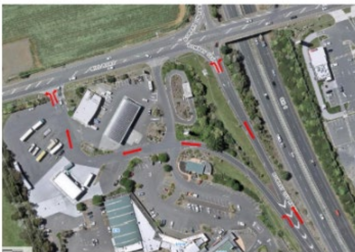
Figure 4 - Illustration of separated left-turn lane before reaching the intersection if queues are present
