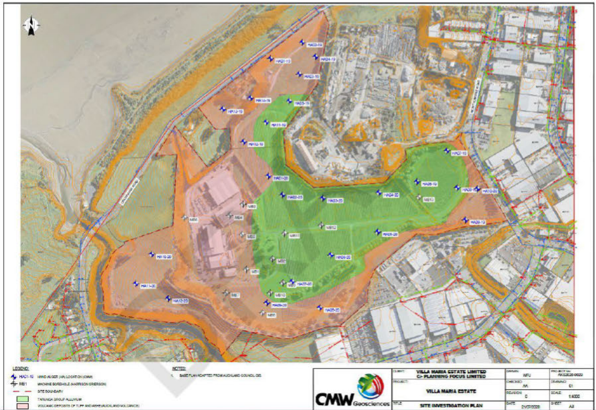
Figure 13: Map showing geotechnical investigations and alluvium (green) and volcanic (red) deposits (source: CMW Geosciences)
