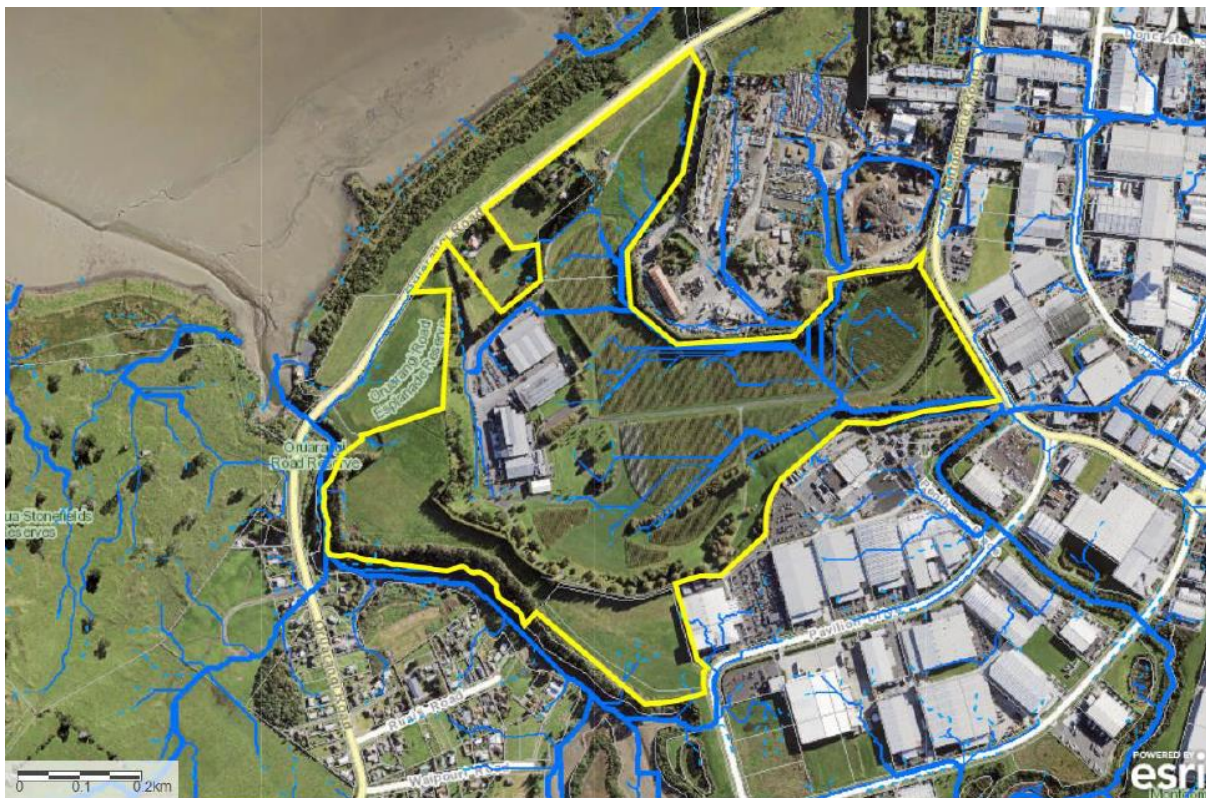
Figure 1. The site at Villa Maria Estate (yellow polygon) and Auckland Council's predicted overland flow paths overlay (blue lines), sourced from Geomaps.
