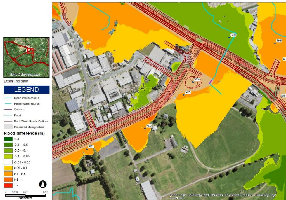
Figure 12-1: Flood Difference Maps for Access Road
