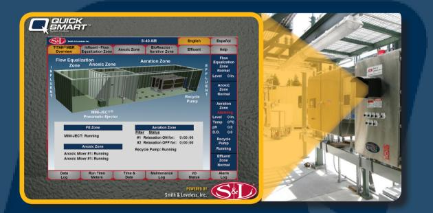
Delivering simplified operation yet powerful TITAN MBR<sup>™</sup> control, QUICKSMART<sup>™</sup> System Controls provide unparalleled ability to monitor and adjust all of your treatment system functions, including:
