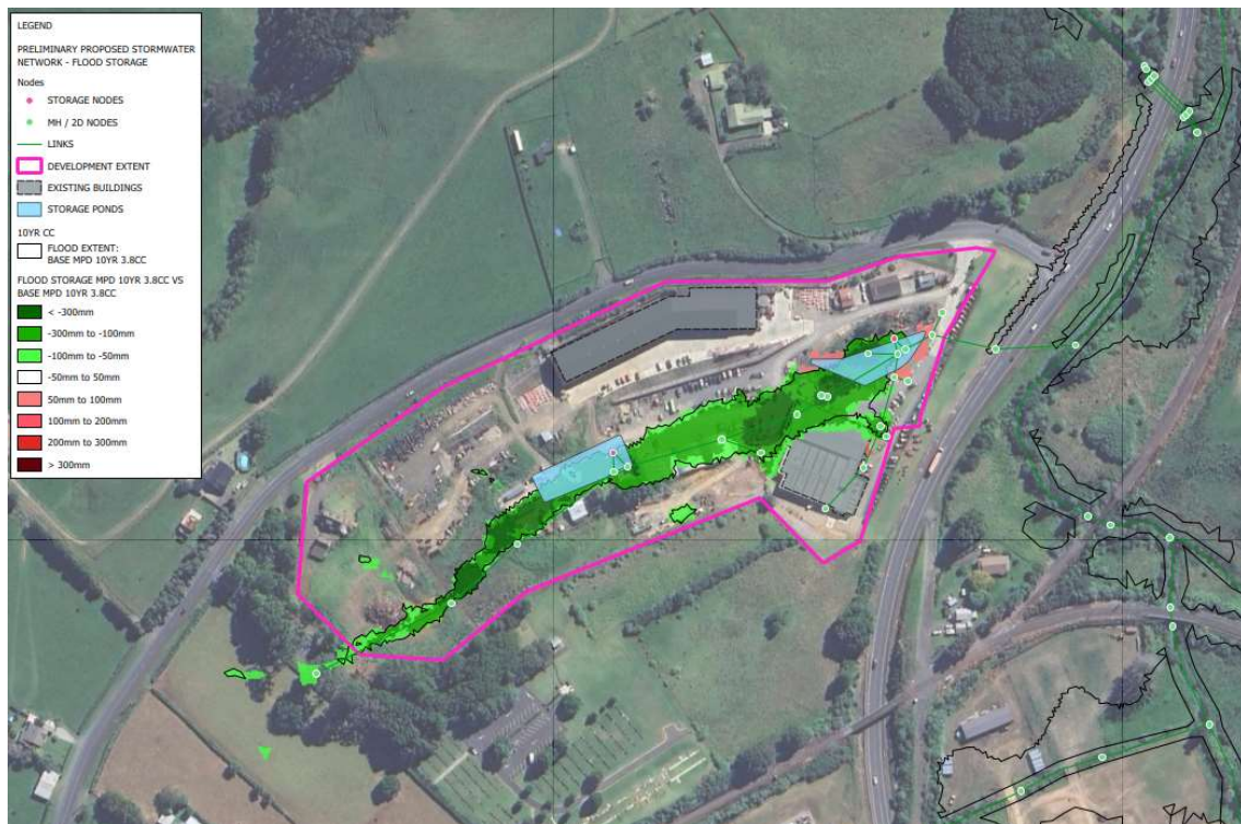
Figure 20: Afflux Plot: Flood Storage MPD with Base MPD (10YR CC + 3.8°C)
