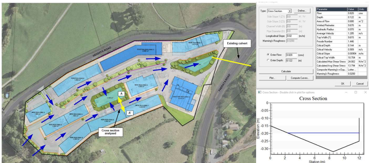
Figure 15: Hydraulic toolbox snippet demonstrating conveyance of external upstream overland flows
