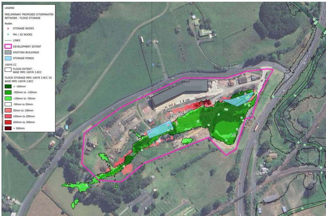
Figure 21: Afflux Plot: Flood Storage MPD with Base MPD (100YR CC + 3.8°C)
