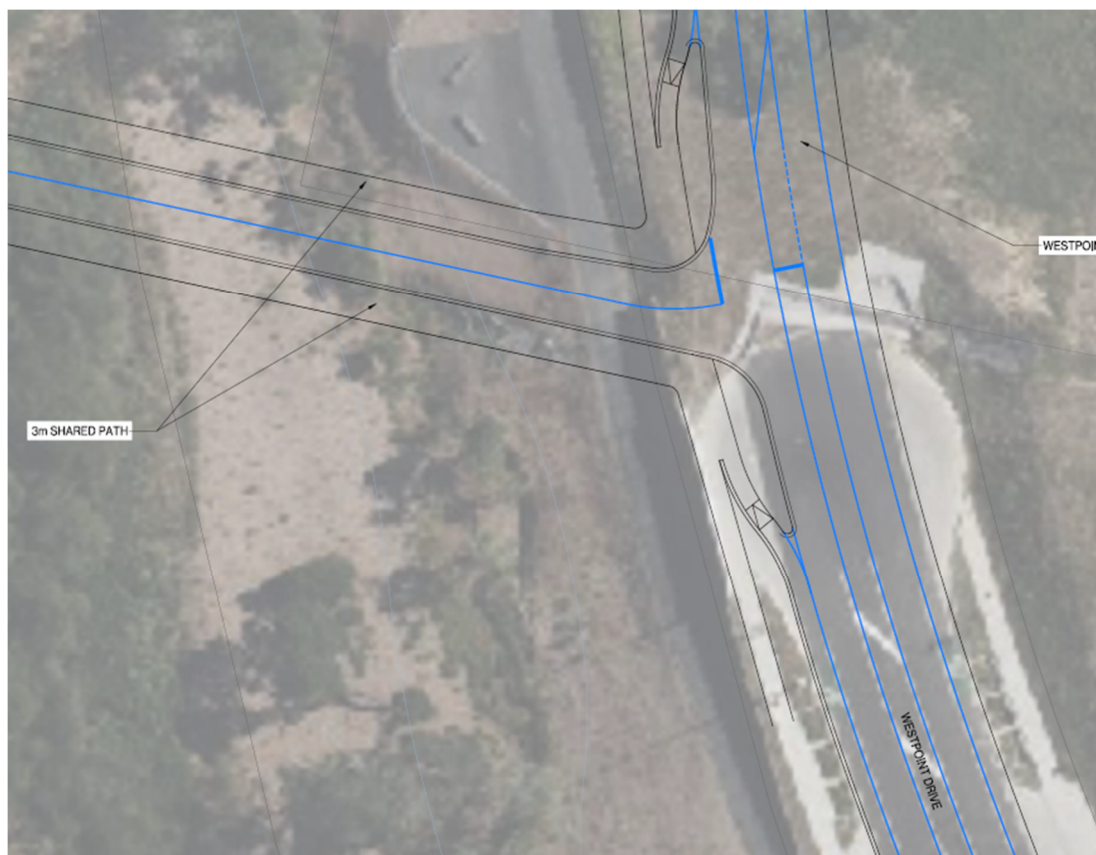
FIGURE 23: BRIDGE/WESTPOINT DRIVE INTERSECTION – CONCEPT DESIGN
