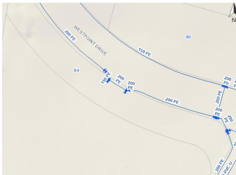
FIGURE 7: CONNECTION FOR FUTURE DEVELOPMENT (SOURCE: AUCKLAND COUNCIL GIS)
