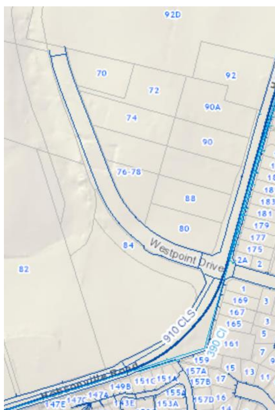
FIGURE 7: EXISTING PUBLIC WATER NETWORK (SOURCE: AUCKLAND COUNCIL GIS)
