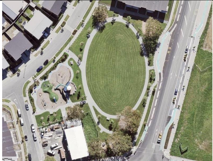
Figure 3: New reserve in Whenuapai, example of assets such as, seating and rubbish bins on perimeter of park to enable a large open space to be achieved in the centre.
