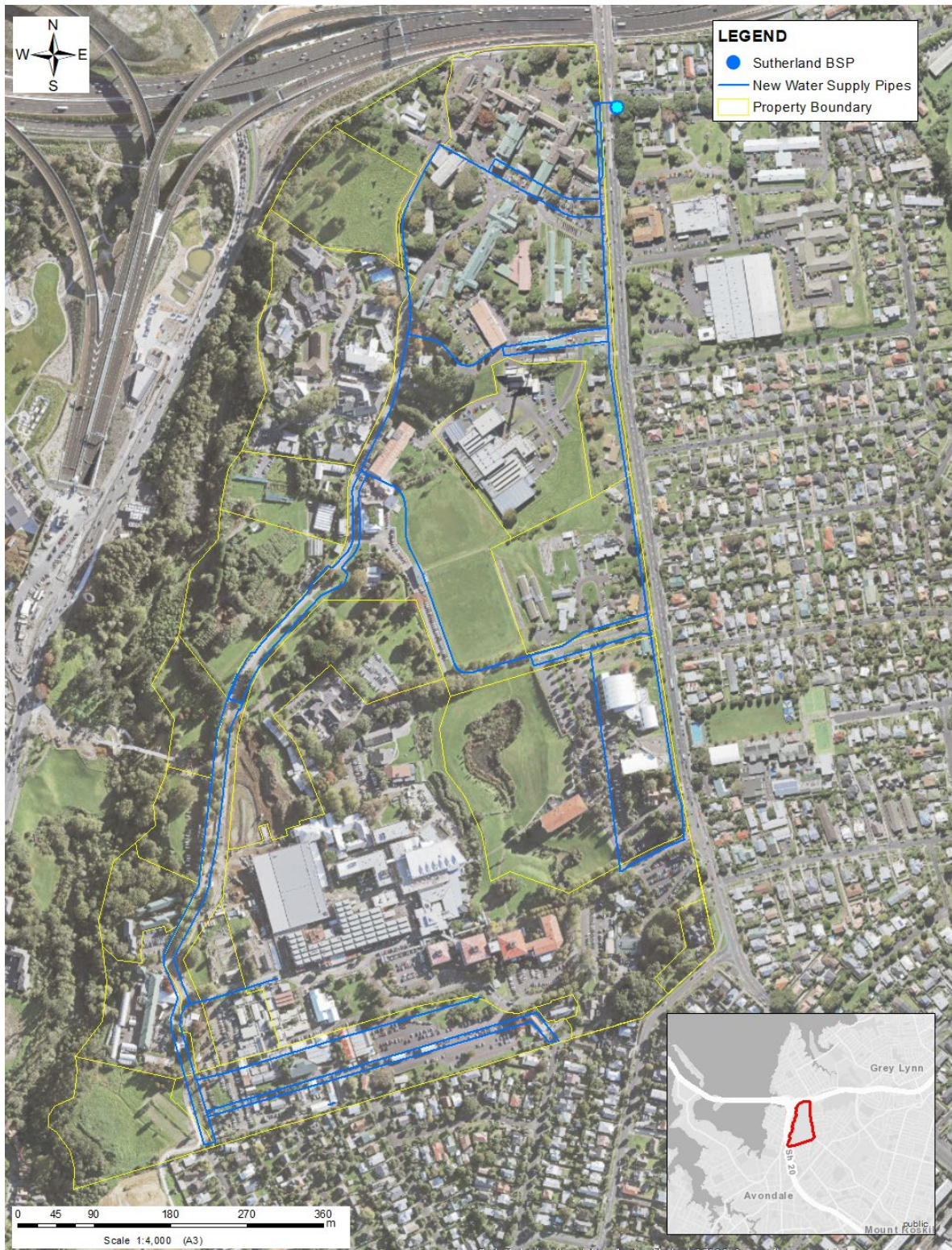
Figure 9 Proposed Water Supply Upgrade Plan
