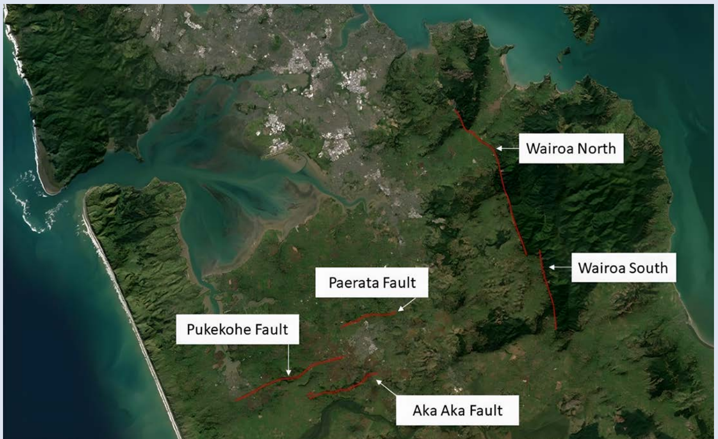
Figure 9: Figure showing faults within the Auckland region (note that the Paerata, Pukekohe and Aka Aka Faults require more research to understand their risks, as recent mapping has just recently identified these features).
