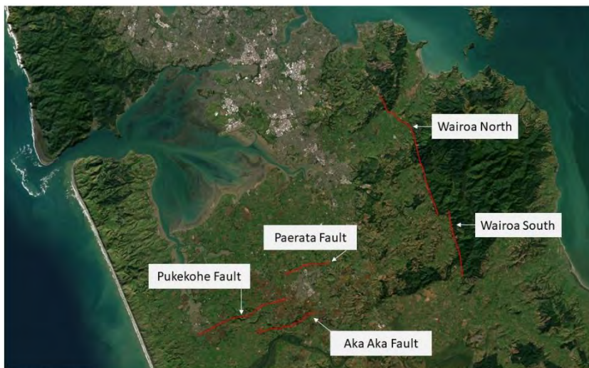
Figure 7 - Figure showing faults within the Auckland region (note that the Paerata, Pukekohe and Aka Aka Faults require more research to understand their risks. as recent mapping has just recently identified these features)
