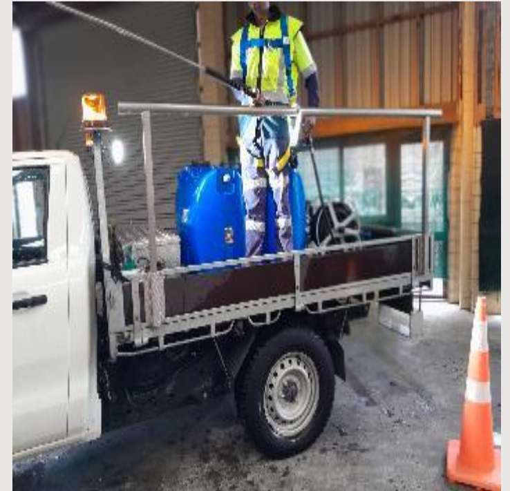
Outfitted the rear section of our water-blasting ute with sturdy safety rails
