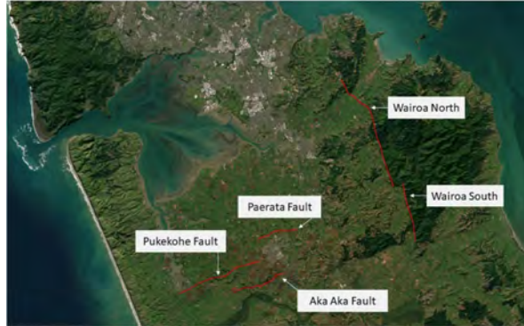
Figure 8 - Figure showing faults within the Auckland region (note that the Paerata, Pukekohe and Aka Aka Faults require more research to understand their risks, as recent mapping has just recently identified these features)
