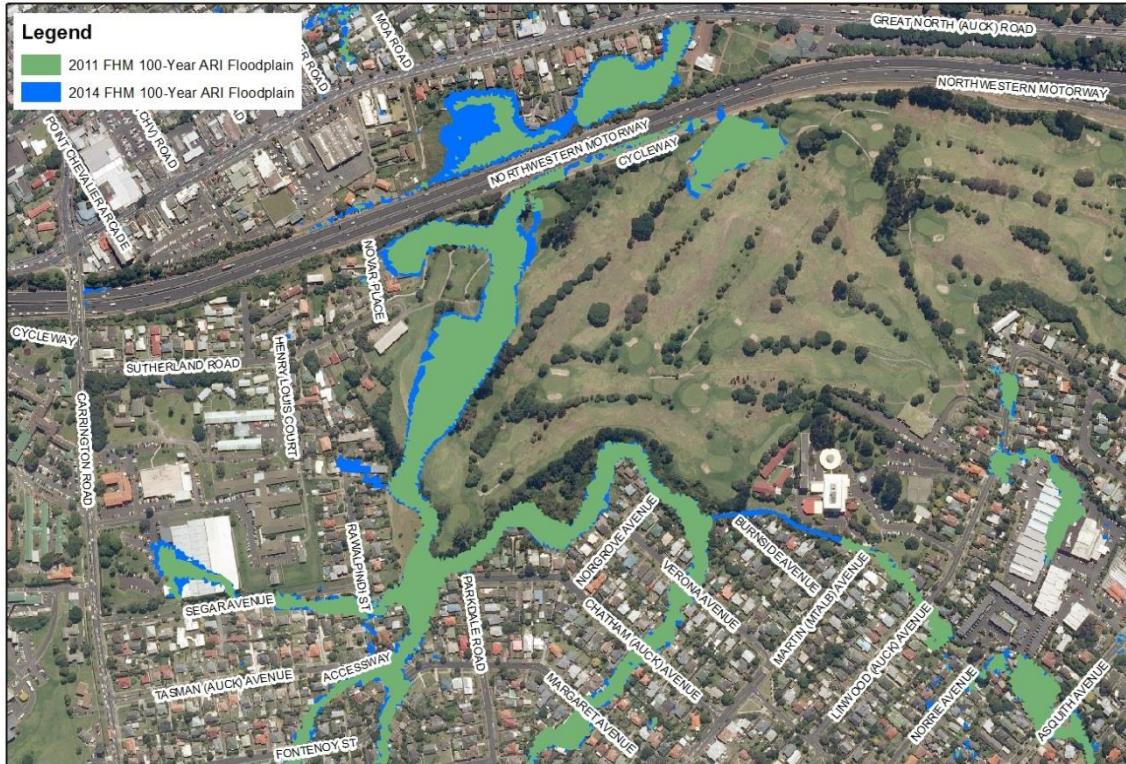
Figure 4-4 Comparison of 100yr ARI MPD Floodplain Extents Upstream of Great North Road
