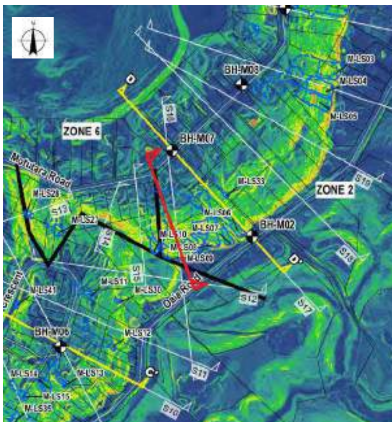
Figure C-2 Assessment area plan indicating the major February 2023 slip areas and the analysed cross-section A-A (retrieved from Google Earth Pro and GHD Atlas). A close-up view of Figure A125 (see Appendix A) showing the analysed cross section 'A' relative to other slope profiles, cross sections and boreholes.
