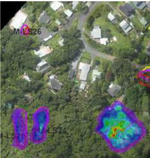
Figure D8 Zone 5 RAMMS calibration using parameters that gives the best match to observed landslide runout
