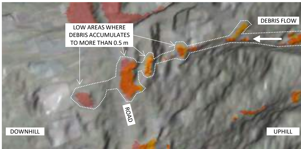
Figure D18 An oblique view of predicted debris flow showing how isolated islands can occur due to the highs and lows of the surface topography.
