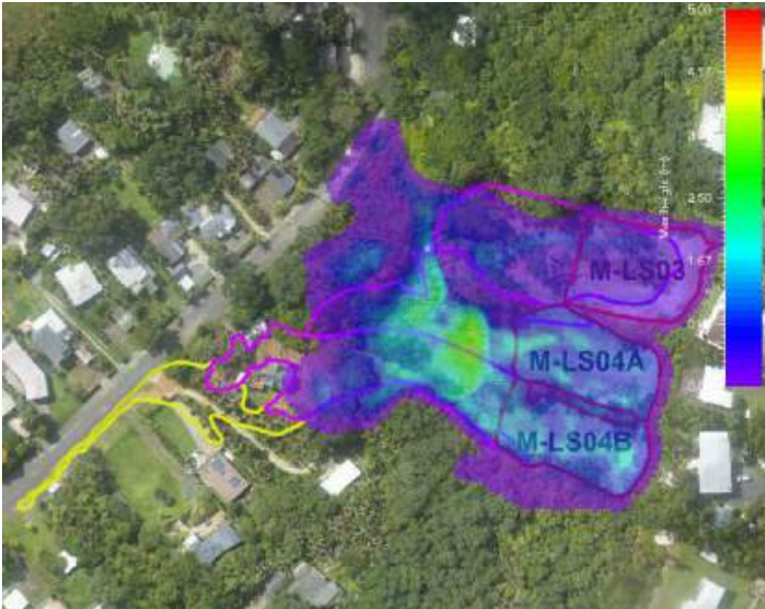
Figure D4 Best calibration of large slides at Motutara Road (M-LS03, M-LS04A and M-LS04B). \mu = 0.225 , \xi = 87.5 , showing with 0.01-5 m filter
