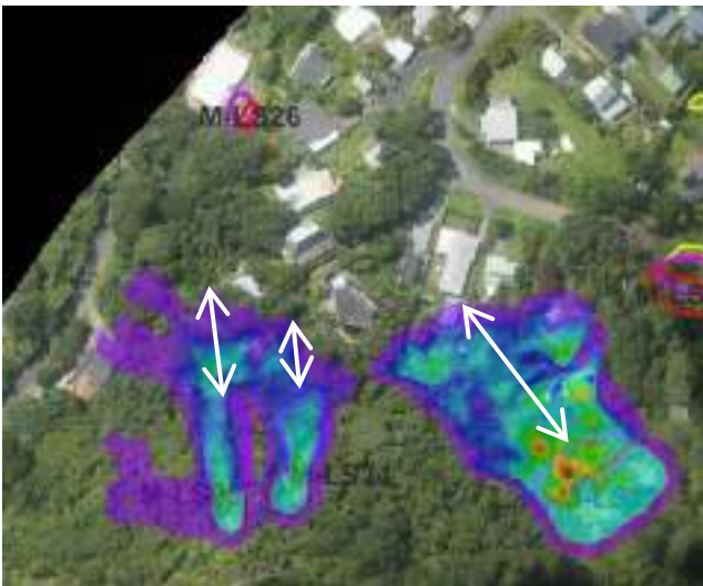
Figure D7 Zone 5 RAMMS simulation showing how the use of (Revision 0) analysis parameters are overly conservative. White arrows show the debris travelling beyond the mapped landslide extents.
