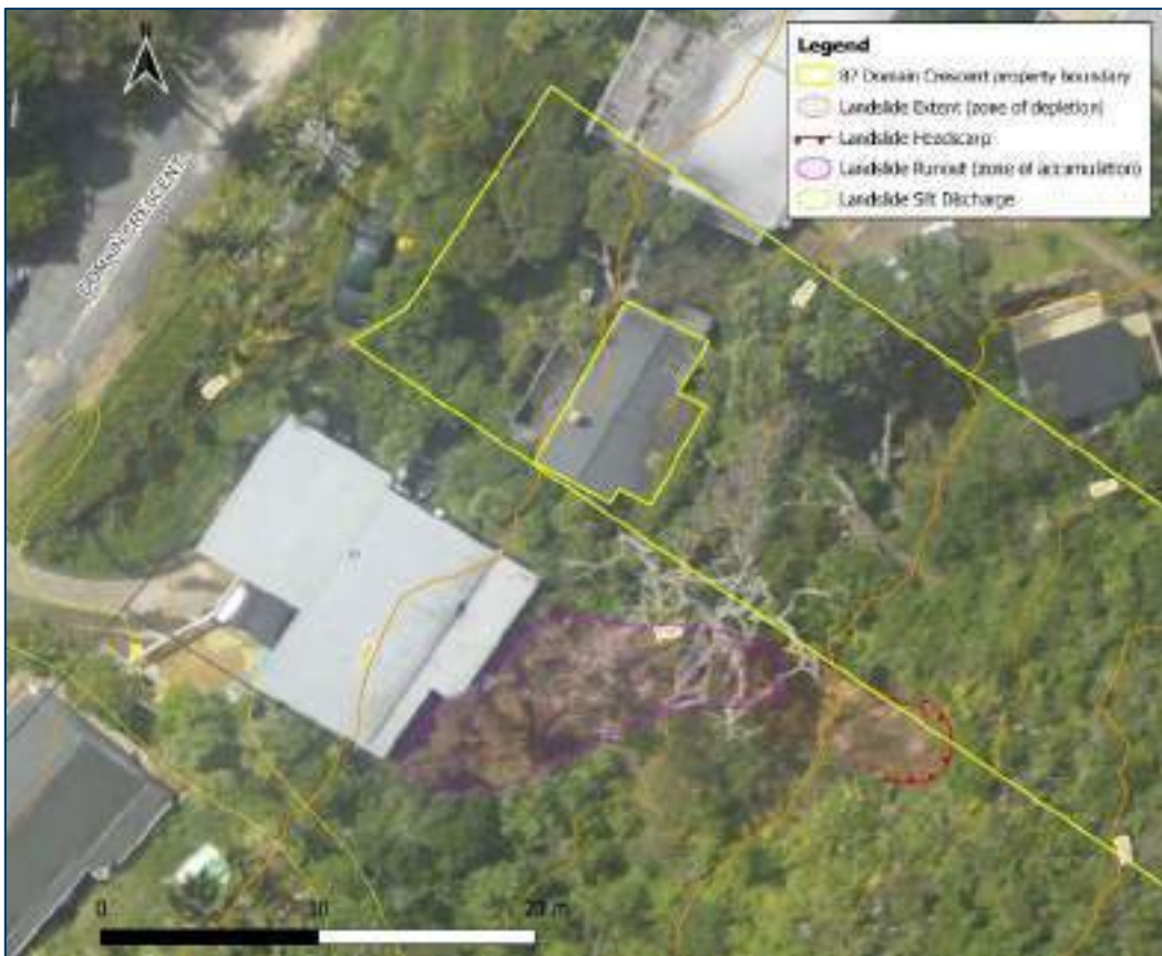
Figure 2.5 GHD site mapping of the landslide affecting the site
