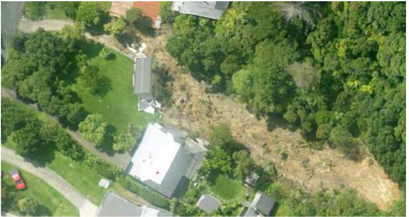
Figure E11 Aerial view of dwelling pictured in Figure E10. The debris flow originated at the far right of the photo.
