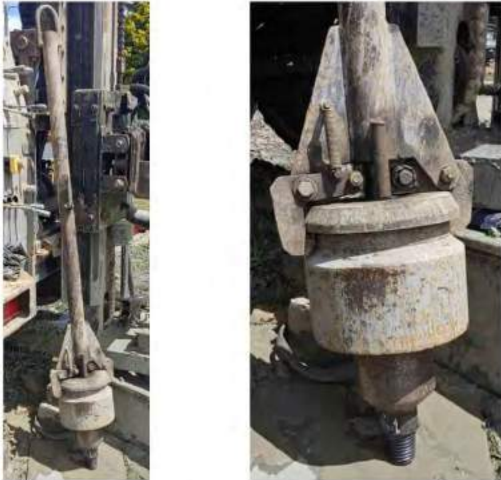
Figure 7-1: Photos of SPT trip hammer #5
