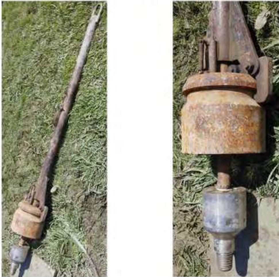
Figure 5-1: Photos of SPT trip hammer #3
