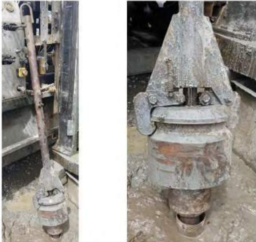
Figure 3-1: Photos of SPT trip hammer #1
