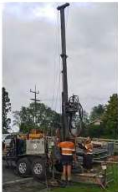
Figure 2-2: Photos of the trailer mounted drill rig and the instrumented SPT rod assembly.
