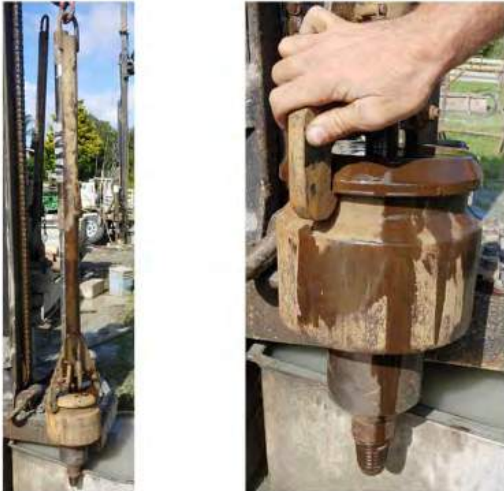
Figure 4-1: Photos of SPT trip hammer #2
