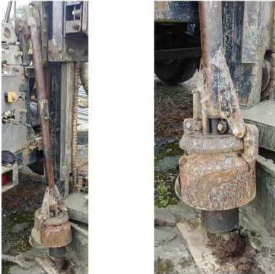
Figure 6-1: Photos of SPT trip hammer #4
