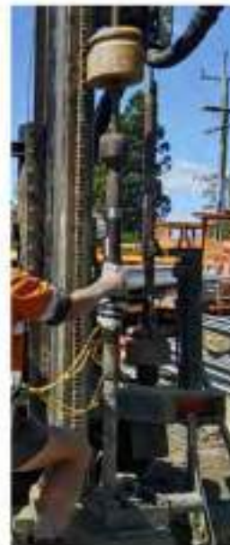
Figure 2-2: Photos of the trailer mounted drill rig and the instrumented SPT rod assembly.
