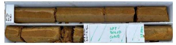
Figure B18 Example of Awhitu Formation Cemented very weak Sandstone, oxidised, from BH-M02 36.65-37.5 mbgl
