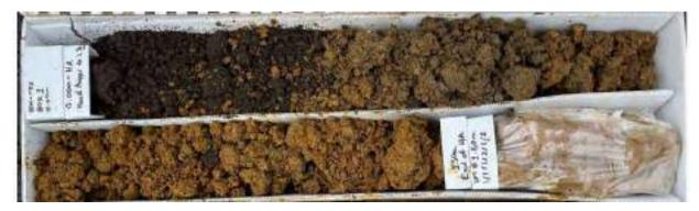
Figure B10 'Fill Deposits' soil recovered in BH - M02: 0.0-1.5 mbgl
