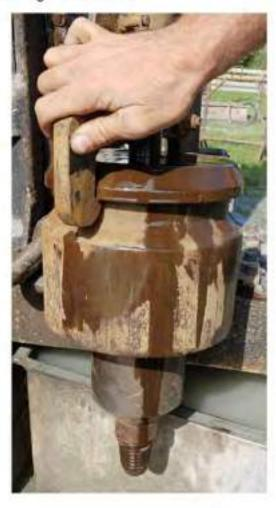
Figure 4-1: Photos of SPT trip hammer #2
