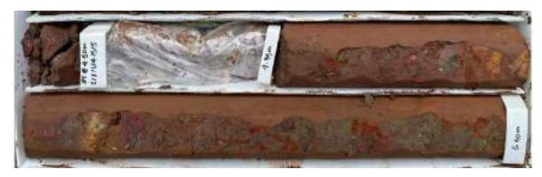
Figure B19 Example of Nihotupu Formation Residual Silt and Clay, from BH-M04 3.95-5.90 mbgl
