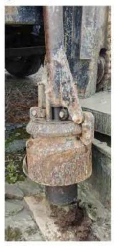
Figure 6-1: Photos of SPT trip hammer #4
