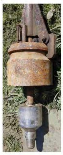
Figure 5-1: Photos of SPT trip hammer #3
