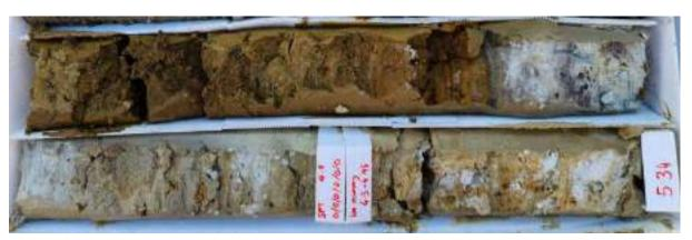
Figure B11 'Ancient Colluvial/Alluvial' soils recovered from BH-M07: 3.65-5.34 mbgl
