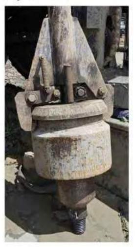
Figure 7-1: Photos of SPT trip hammer #5
