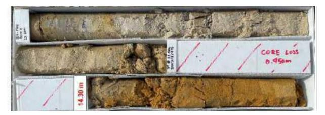
Figure B14 Example of Awhitu Formation Less Cemented Sands, weakly consolidated material from BH-M02, 11.6-14.7 mbgl
