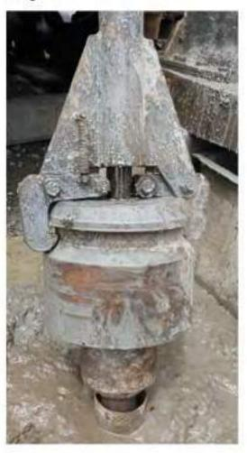
Figure 3-1: Photos of SPT trip hammer #1
