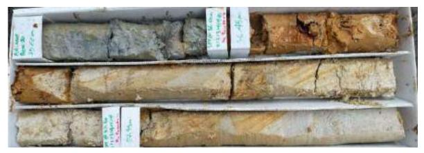
Figure B12 Example of in-situ 'blocks' of cross-bedded Awhitu Formation within Ancient Colluvial/Alluvial soils, from BH-M06: 36.45-38.2 mbgl
