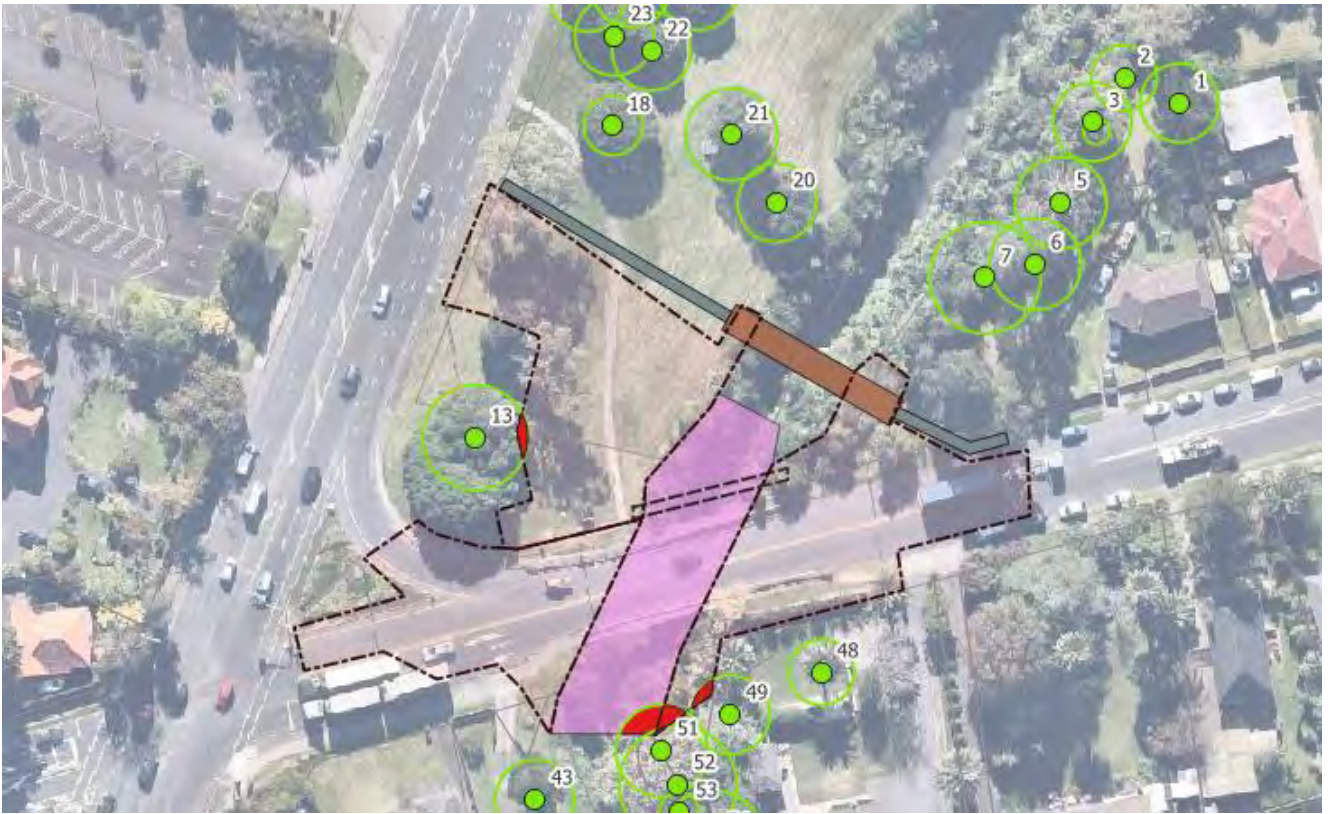
Figure 4: A screenshot from a geospatial analysis depicting protected root zone (green circles around trees) incursions (red areas).
