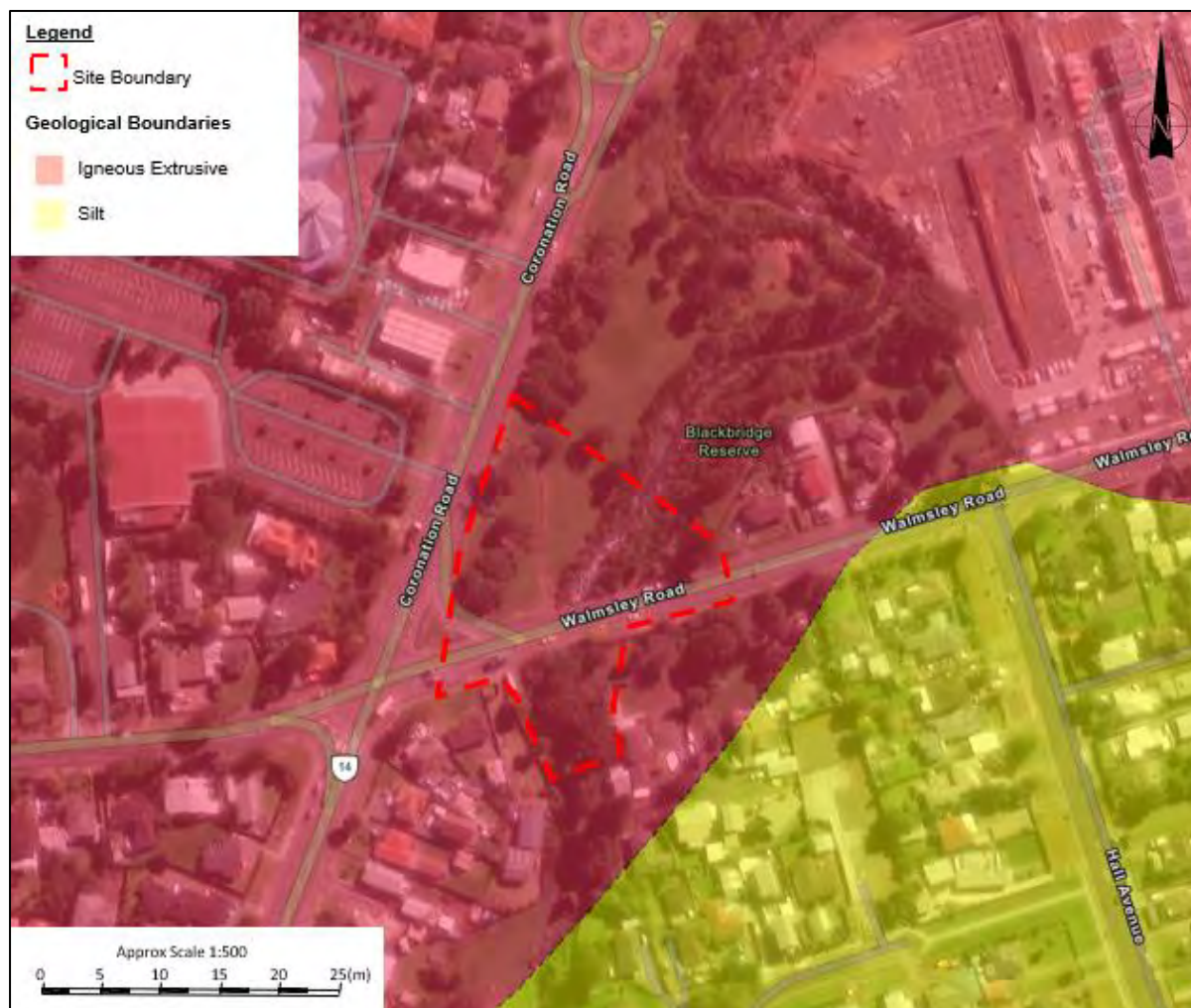
Figure 2.1: Published geological map in relation to the project area (Source T+T Map Viewer 6 ).
